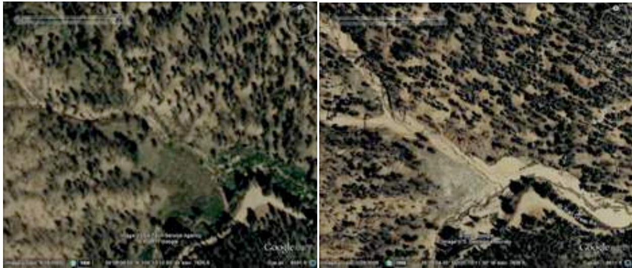
Google Earth photos of Trail Creek drainage. Photo on left taken in 2003, the year after the fire. The same drainage, on right, after a flood event in 2006, showing large areas of sediment deposition.
