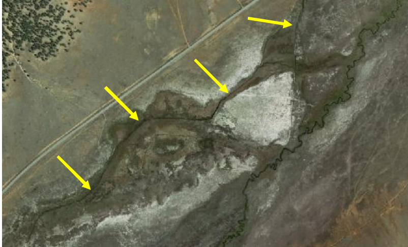
Figure 5: The ditch line identified by the arrows was constructed around 1970 with the apparent purpose of draining riparian wetland area along Fourmile Creek near Hartsel.
